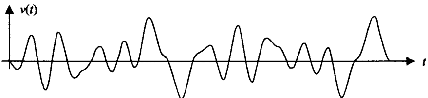
Figure 6.22. Seven-tone multitone created with random phases.
