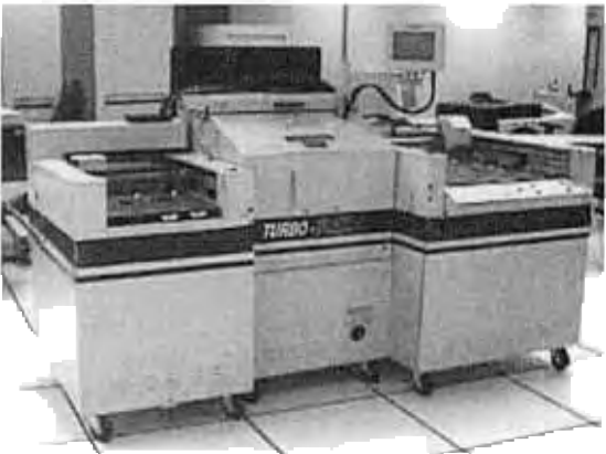
Figure 1.16. Delta robotic handler.
